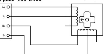
One pole of each winding and the centre tap are connected the other pole of each winding should be taped off and isolated.
